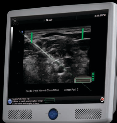
SonixGPS helps to accurately predict your needle's trajectory
